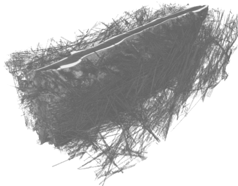
Membrane electrode assembly of a used PEM fuel cell (thickness 700 \mu\text{m} ) imaged by x-ray computed tomography.
