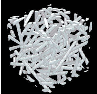
Fig. 1. Realization of a random fiber system with isotropic orientation, filling factor 10 %.
