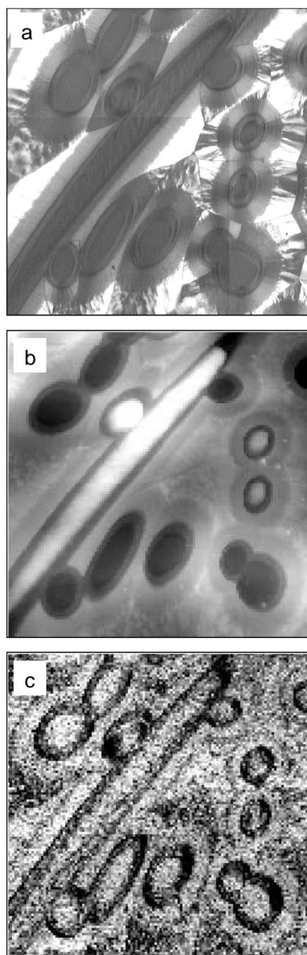
Fig. 1. Micrographs of a cross-sectional area of a carbon infiltrated carbon felt taken by (a) polarized light microscopy (PLM), (b) atomic force microscopy (AFM, topography) and (c) pulsed force microscopy (PFM).
